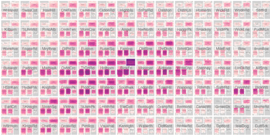
Fig. 7.12 Represents the density of moving vehicles in London, by grid square, day of week, hour of day and vehicle type, using a logarithmic colour scale. Figure based on Slingsby et al. (2010) with permission from the original authors
