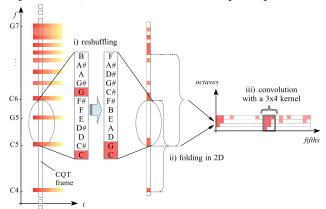
**Figure** 2. *F-CQT* example for a C4 note: (i) each CQT frame is reshuffled on an octave-per-octave basis, folded (ii) using 2-octave wide half-overlapping bands, in order to avoid side effects. A kernel (iii) of size 12 captures 8 out of the first 12 harmonics including the fundamental.
