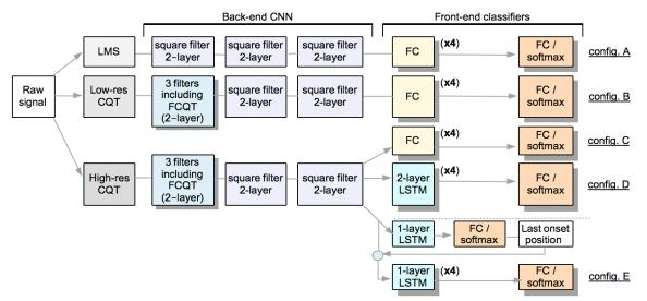
**Figure 1.** System architecture (incremental configurations A to E). A is directly inspired by [11]. B introduces CQT along with adapted filtering in the convolutional process. The resolution of CQT is increased in C. Recurrent layers process the output of the CNN in D. Finally, in configuration E, we experiment with the joint classification of onsets.
