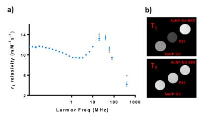
**Figure 1.** Relaxometric and MRI studies of AuNP-Gd and AuNP-Gd-BBN particles: (a)  $^1$ H NMRD profiles of AuNP-Gd (•) and AuNP-Gd-BBN (•) (25 °C); (b)  $T_1$ - and  $T_2$ -weighted MRI phantom images obtained at 9.4T (25 °C): [Gd]<sub>AuNP-Gd</sub> = 0.25 mM and [Gd]<sub>AuNP-Gd-BBN</sub> = 0.22 mM.
