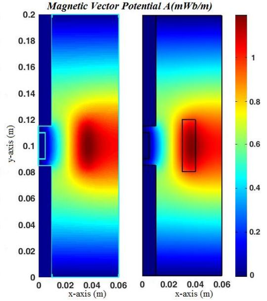
Fig.2. Comparison of the distributions of the magnetic vector potential obtained from the analytical calculation (on the left) and the numerical calculation (on the right).
