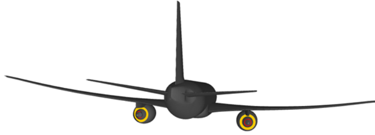
Figure 2: Modified CRM wing/body/engine configuration, highlighting engine primary core (red) and bypass flow (orange)
