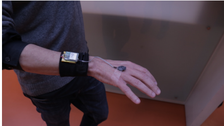
Sidebar 2: RIoT sensor with a detached IMU sensor.
