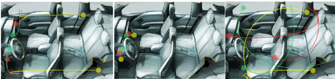
Figure 2 – Depiction of the spatialisation concepts of the three driving modes of Symbioz: natural for Classic (left), focused for Tonic (middle), diffused for Autonomous (right)
