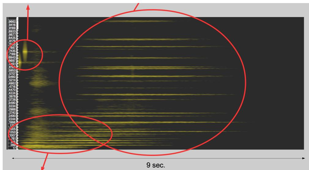
Figure 3 – Sonogram of *AD Definitive* HMI (from left to right red circles ○): *brain sounds* reminding AD mode setting; sound confirming successful locking in AD mode; multisense sound reinforcing light design.
