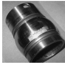
Fig. 25. Inner race fault observed in bearing 3.
