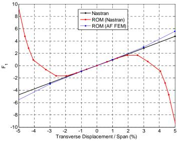
Figure 2. Modal force along mode 1 vs. tip transverse displacement for a flat cantilevered beam. Results from Nastran nonlinear static (SOL 106), the ROM identified from the Nastran model ("ROM(Nastran)") and from the Air Force code Bobtran ("ROM(AF FEM)") implementing [13].
