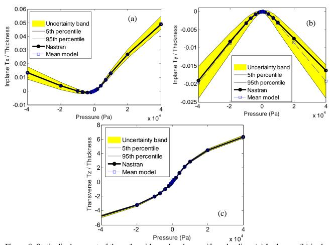
Figure 8. Static displacement of the orthogrid panel under a uniform loading. (a) Inplane x, (b) inplane y, and (c) transverse z displacements at a quarter point divided by the panel thickness vs. load. Mean and uncertain models.
