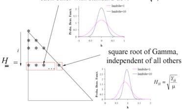
Figure 1. Structure of the random *H* matrices with n = 8, i = 2, and  $\lambda_0 = 1$  and 10.
