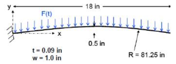
Figure 5. Cantilevered curved beam with uniform loading.
