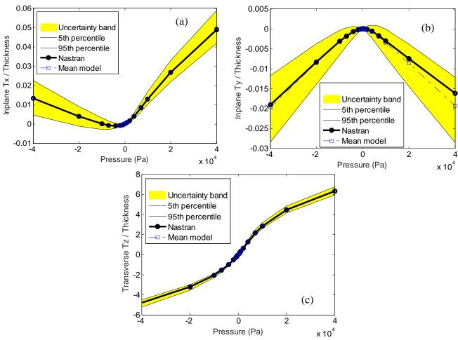
Figure 12. Static displacement of the orthogrid panel under a uniform loading. (a) Inplane x, (b) inplane y, and (c) transverse z displacements at a quarter point divided by the panel thickness vs. load. Mean and uncertain models, approach of section 5.5.
