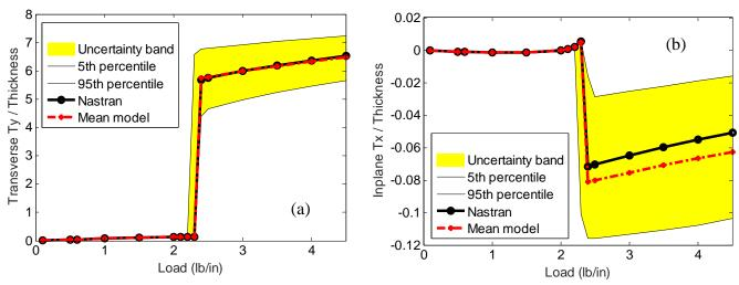
Figure 11. Static displacement of the clamped-clamped curved beam under a uniform loading. (a) Transverse and (b) inplane displacements (in percent of span) of a beam quarter point vs. load. Mean and uncertain models, approach of section 5.5.
