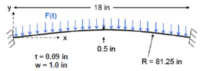
Figure 9. Clamped-clamped curved beam with uniform loading.
