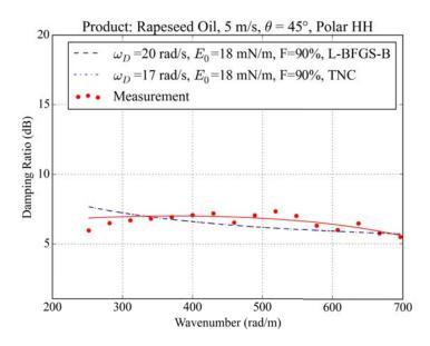
**Figure 15.** Damping ratios calculated for rapeseed oil slick by considering a wind speed of  $5\,\mathrm{m/s}$  in HH polarization for an incidence angle of  $45^\circ$ . The data points (red dots) are fitted by a third-degree polynomial (red line). The dashed lines are the damping ratios obtained from the minimization process (black dashed line: L-BFGS-B method, blue dotted line: TNC method).
