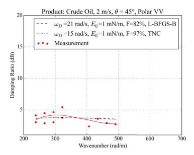
**Figure 14.** Damping ratios calculated for crude oil spill by considering a wind speed of  $2 \,\mathrm{m/s}$  in VV polarization for an incidence angle of  $45^\circ$ . The data points (red dots) are fitted by a third-degree polynomial (red line). The dashed lines are the damping ratios obtained from the minimization process (black dashed line: L-BFGS-B method, blue dotted line: TNC method).
