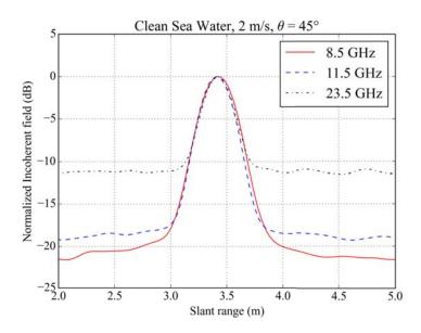
**Figure A1.** Normalized incoherent field of the clean seawater surface with an incidence angle  $45^{\circ}$  and a wind speed of  $2 \,\mathrm{m/s}$  in VV polarization. Three EM frequencies are shown:  $8.5 \,\mathrm{GHz}$  (red line),  $11.5 \,\mathrm{GHz}$  (blue dashed line) and  $23.5 \,\mathrm{GHz}$  (black dotted line).
