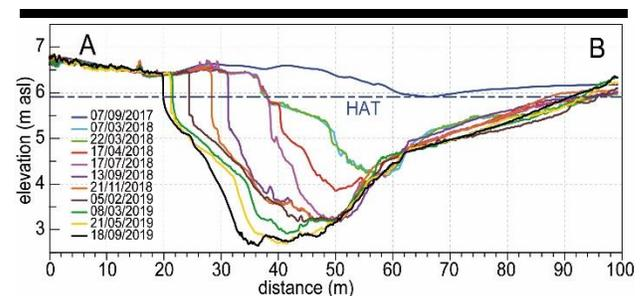
Figure 7. Deepening and widening of the breach from March 2018 to September 2019 (see transect location on Figure 6).
