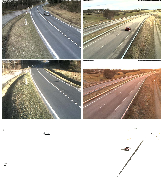
Fig. 4. Guided Image Difference operator applied on two image pairs. The output is shown in the third line after a morphological opening and a thresholding.
