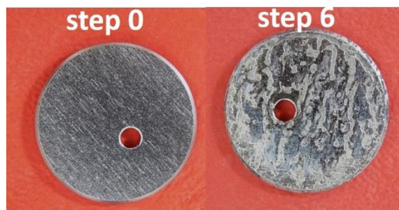
Fig. 5.- Macrographs of the surfaces of aluminized René 125 before and after 6 steps (alternated cathodic and anodic polarizations).
