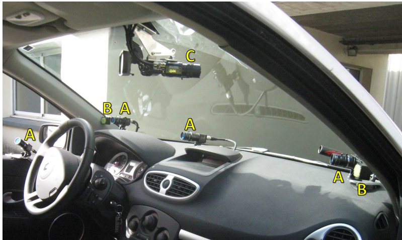
Figure 2: Photograph of the instrumented vehicle. A: Cameras to collect gaze information. B: Infra-red lamps. C: Scene cameras.
