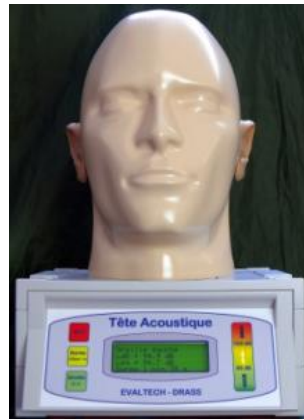
Figure 3: Acoustic head used for measuring acoustic level of music players. Initial green light becomes orange above 85 dBA, for one ear, and red above 100 dBA
