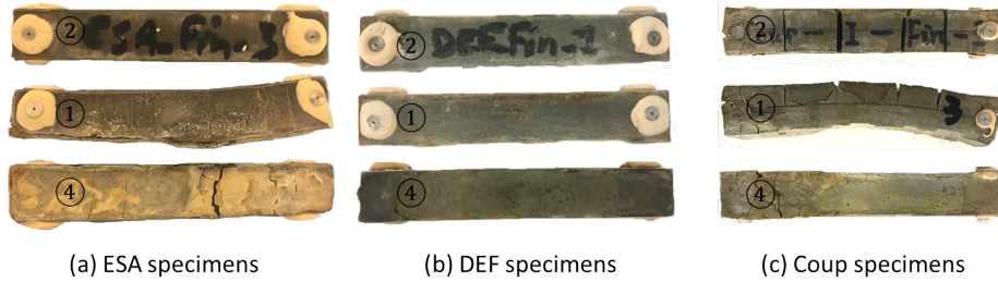
Figure 5: Observations of (a) ESA specimens after 7 months; (b) DEF specimens after 2 years; and (c) Coup specimens after 2.5 months on faces 1, 2 and 4.
