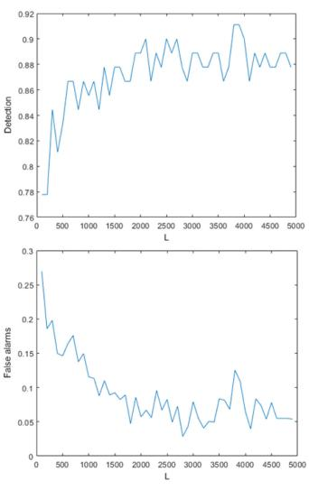
**Fig. 7.** Values of  $P_D$  (top) and  $P_{FA}$  (bottom) versus the number of dictionary atoms L.
