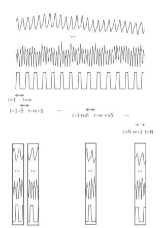
Fig. 2. Segmentation of telemetry into overlapping windows.
