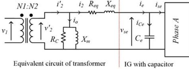
Fig. 4. Equivalent circuit of transformer and IG
