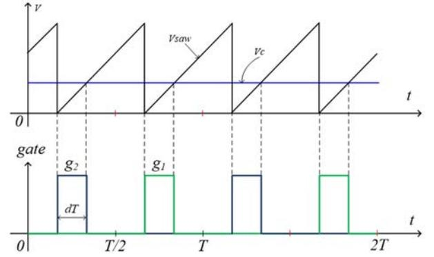
Fig. 5. Gate signal for T1 and T2 MOSFETs of the UPS
