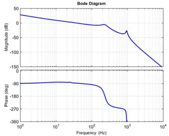
Fig. 13. Overall open loop frequency response of  $T(s)$
