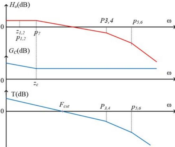
Fig. 8. Asymptotic Bode plots for controller design
