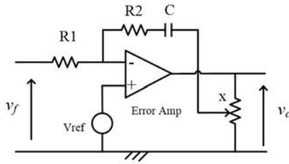
Fig. 7. PI Controller with error amplifier
