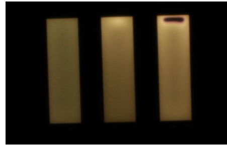
Fig. 2. Catastrophic degradation under strong current (carbonization area appearance)
