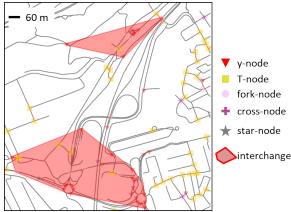
Figure 10: Vector-based detection algorithm used on the roads extracted from an image classified as highway interchange: the interchange is detected but with two different parts, the middle sections being left undetected.
