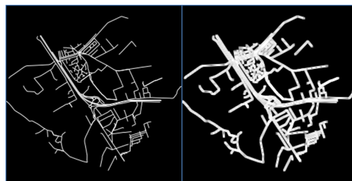
Figure 17: Two images generated with a road symbol width of 1 pixel on the left and 2 pixels on the right.
