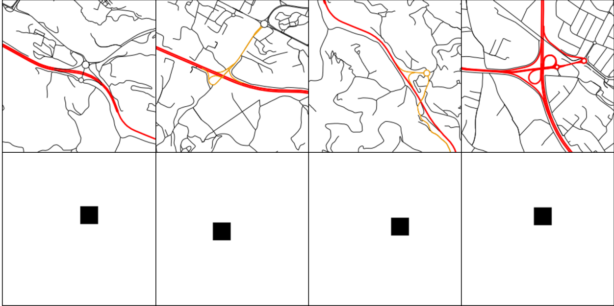
Figure 12: Four examples used to train the segmentation model. In the input images on top, the colors are related to the importance value of each section (red is most important, and black is least important). In the label images below, a black square is generated around the interchange points.
