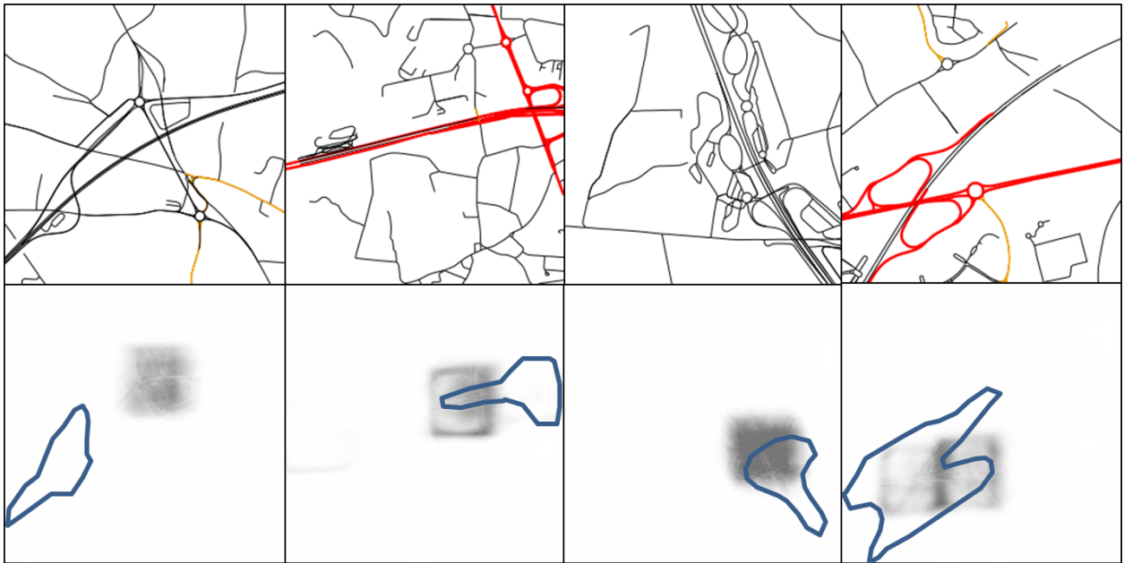
Figure 15: Results of segmentation compared with handdrawn interchange delineation.
