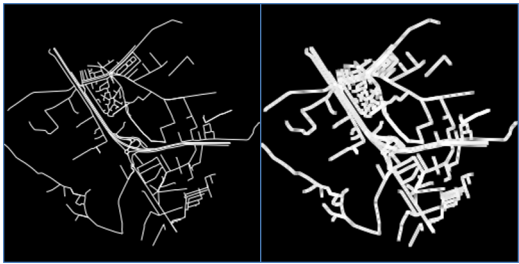
Figure 17: Two images generated with a road symbol width of 1 pixel on the left and 2 pixels on the right.
