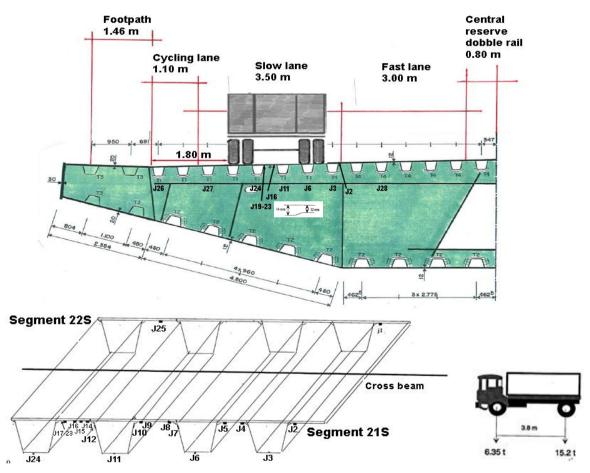
Figure 2 – Bridge of Normandy, transverse cross section, stain gauges and test truck (1995)
