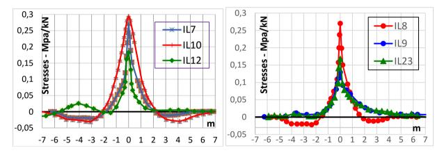
Figure 3 – Influence lines: stiffener flange (left), upper plate/deck (right)
