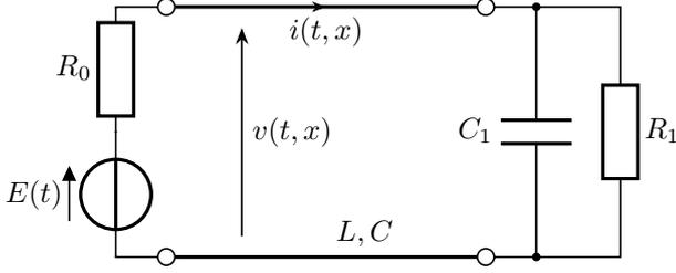
Fig. 1. Electrical circuit with a transmission line
