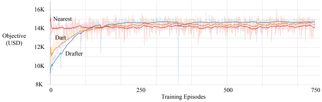
Figure 5: Training curves for the Dart (orange) and Drafter (blue) agents over 750 training instances of size 1400/43. Nearest (red) is provided as a reference. Darker curves are smoothed representations of the lighter curves.
