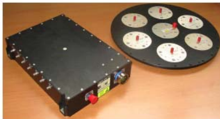
Fig. 4 7-element antenna array and associated electronics
