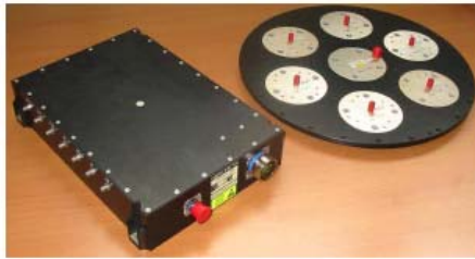
Fig. 4 7-element antenna array and associated electronics
