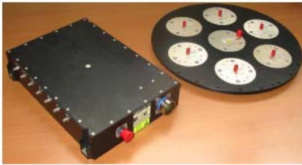
Fig. 4 7-element antenna array and associated electronics
