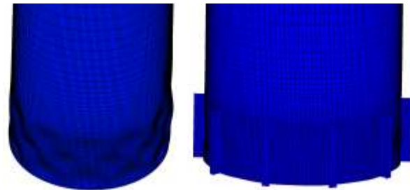
(a) without stiffeners (b) with 10 HEA 180 stiffeners
