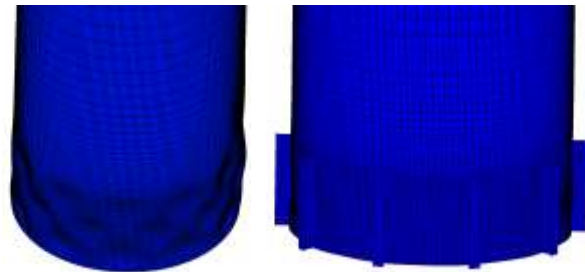
(a) without stiffeners (b) with 10 HEA 180 stiffeners
