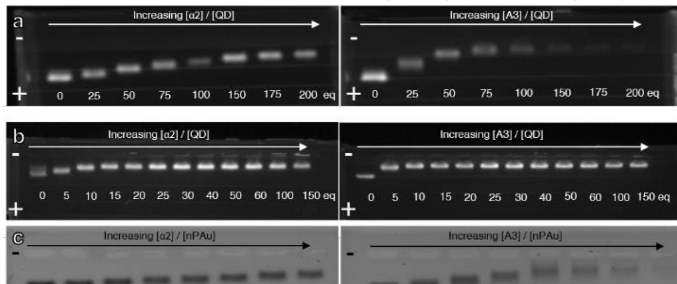
**Fig. 2** Agarose gel electrophoresis of peptide-stabilized (a) 9-nm QD<sup>655</sup>, (b) 2.5-nm QD<sup>545</sup> and (c) 8-nm AuNP incubated with increasing amounts of  $\alpha 2$  (left) or  $\alpha 3$  (right). The buffer used is at pH 8.
