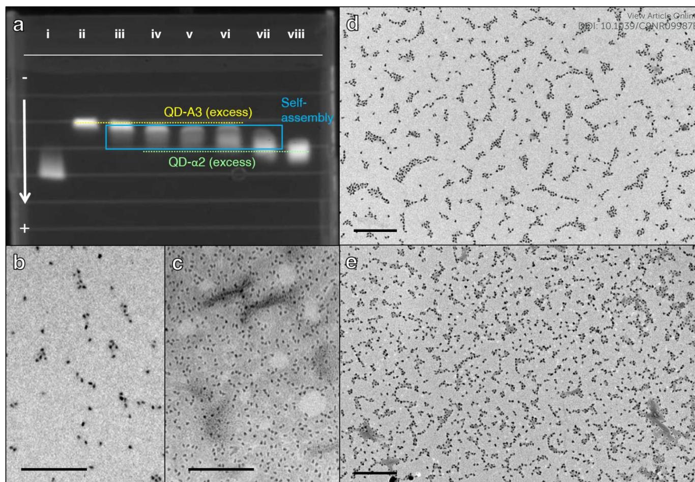
**Fig. 4** (a) Fluorescence image of the agarose gel electrophoresis of pure QD-C5PEG4, QD-A3, mixtures of QD-A3 and QD- $\alpha$ 2 at 5:1, 2:1, 1:1, 1:2 and 1:5 molar ratios respectively and QD- $\alpha$ 2 in tracks i–viii respectively. TEM images of (b) pure QD-A3, (c) pure QD- $\alpha$ 2, (d) 1:1 QD- $\alpha$ 2 + QD-A3 mixture and (e) 1:5 QD- $\alpha$ 2 + QD-A3 mixture. Scale bars represent 100 nm.
