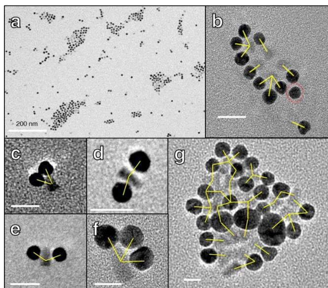
**Fig. 6** TEM images of (a) large self-assemblies of QD-A3 and AuNP- $\alpha$ 2 and (b-g) spatially limited self-assemblies QD-A3 and AuNP- $\alpha$ 2. Scale bar is  $20 \text{ nm}$  for B and D. Scale bar is  $10 \text{ nm}$  for C. Yellow bars represent QD-AuNP pairs that are possibly linked by protein pairs. Red dotted circle indicates AuNP with no obvious link to QD.
