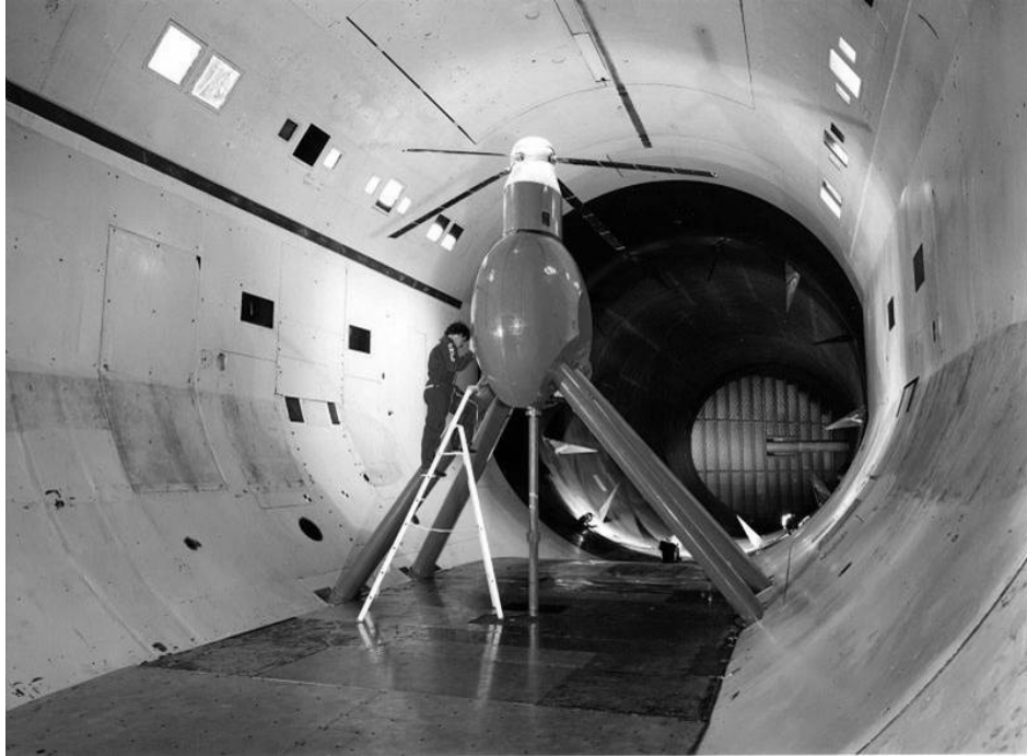
Fig. 1: 7A rotor mounted in ONERA Modane S1MA wind tunnel.
