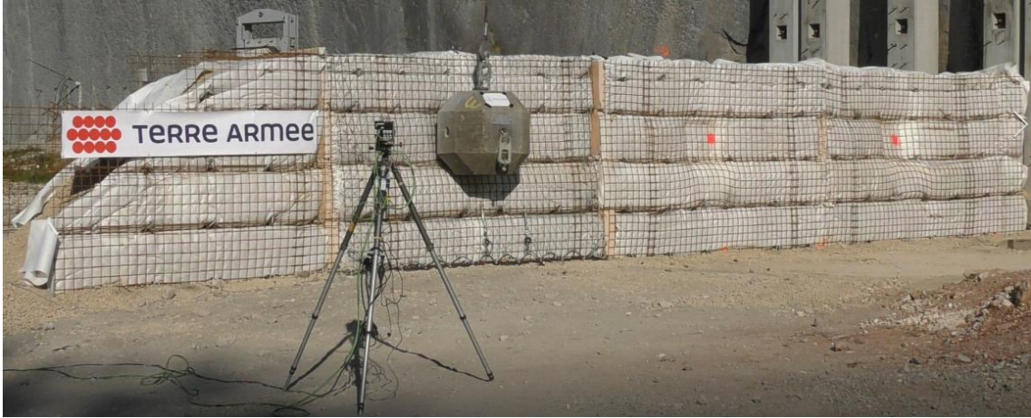
Figure 4. Front face view of all the bunds after the first impact.
