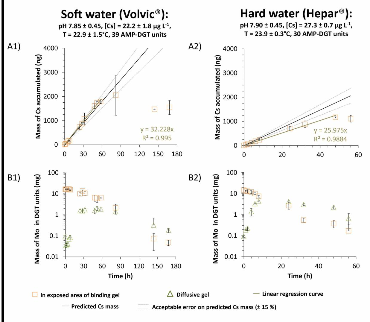
Results of time-series experiments performed with APA diffusive gel in soft and hard waters:
