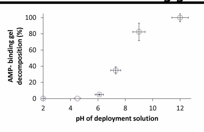
Stability investigation of AMP-binding gelduring 21 h of deployment time in 20 mL of  $10^{-2}$  mol L<sup>-1</sup> NaNO<sub>3</sub> solution at various pH (2–12).
