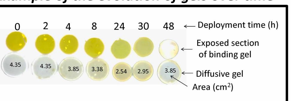
The change in color of AMP binding gel and the shape evolution of APA diffusive gel (only observed in hard water) over time.
