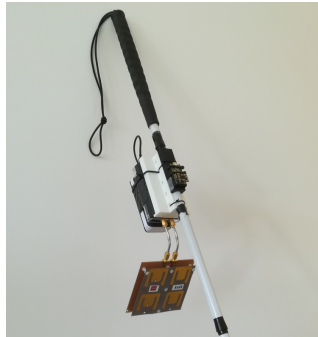
Fig. 10: Prototype of the electronic white cane
