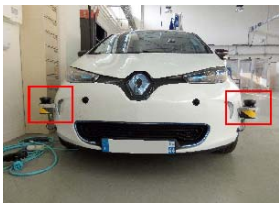
LiDARs installed on the front
