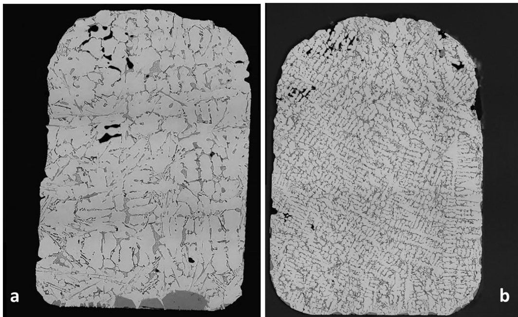
Fig. 3. Mosaic image of LOM micrographs of the samples cooled at 0.5 °C/min (a) and 5 °C/min (b). The width of the sample section is 3.9 mm.
