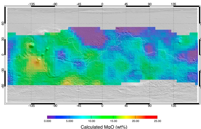
**Figure 7.** Concentration of MgO at the surface of Mars calculated by difference from GRS geochemical maps for FeO, Al<sub>2</sub>O<sub>3</sub>, CaO, SiO<sub>2</sub>, K<sub>2</sub>O and elemental ratios in Martian meteorites for other major oxides (P<sub>2</sub>O<sub>5</sub>, TiO<sub>2</sub>, Na<sub>2</sub>O, MnO). The dotted white line represents the dichotomy boundary defined from crustal thickness [Watters *et al.*, 2007].
