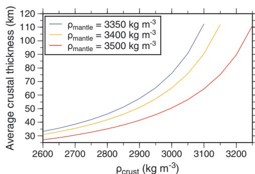
**Figure 15.** Average crustal thickness as a function of crustal density for three different mantle densities. For each crustal thickness inversion, the minimum crustal thickness was constrained to equal 1 km.
