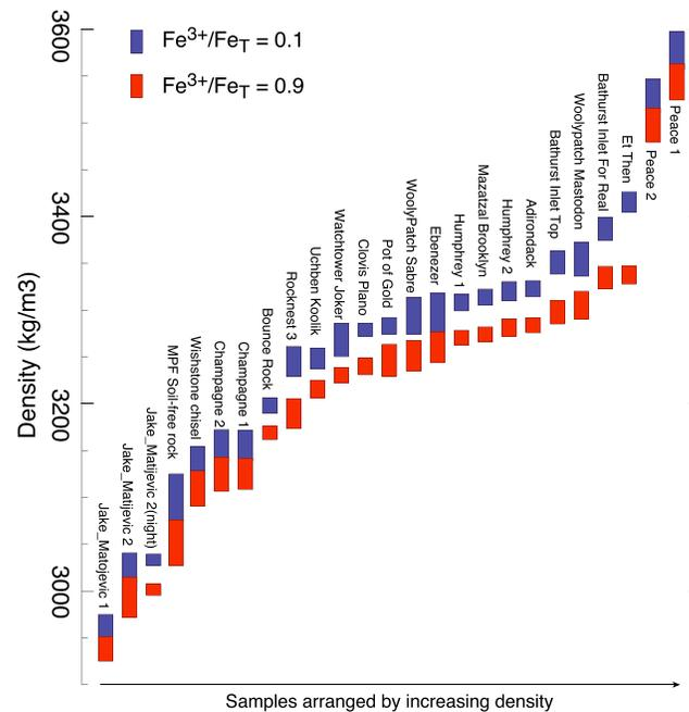
**Figure 5.** Density of igneous rocks at Mars Pathfinder landing site (MPF soil-free rocks), Gale crater (Jake Matijevic, Bathurst Inlet, Et Then, Rocknest 3), Meridiani (Bounce rock), and Gusev crater (all others data) estimated from CIPW norm and APXS S-free and Cl-free measurements. Rocks were cleaned using the Rock Abrasion Tool of the Mars Exploration Rovers for Gusev Crater and Meridiani. Density is calculated for two extreme conditions of oxidations.
