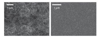
**Figure 3** SEM micrographs without (left) and with (right) metallization of an 8-bilayer film (16.5 nm/bilayer, R = 2%). The CNCs are clearly visible as rigid rods after the metallization step, while the SWNTs are visible without the metallization thanks to their conducting properties (entangled bright structures).
