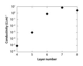
**Figure 5** Conductivity of an 8-bilayer film (16.5 nm/bilayer) when only the numbered bilayer is composed of SWNT/CNC hybrids (f = 11.2%), the other ones being without SWNTs. Layer number 1 is at the bottom and layer number 8 is the top layer.
