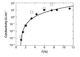
**Figure 4** Conductivity of 8-bilayer films versus the fraction *f* of SWNTs. The black diamonds show the 16.5 nm/bilayer thick films (built in the presence of salt) and the white squares the 8.8 nm/bilayer thick one, respectively. The continuous line shows the fit of the black diamonds with a percolation law as discussed in the text.
