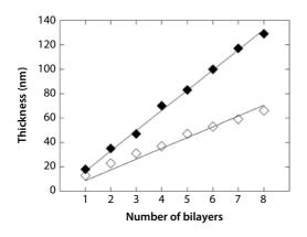
**Figure 2** Thickness of the thin films versus number of deposited bilayers (R = 2%). The black diamonds show the growth in the presence of 1M NaCl, the white diamonds correspond to the films obtained without NaCl. The straight lines give an average thickness of 16.5 nm/bilayer and 8.8 nm/bilayer with or without salt respectively.
