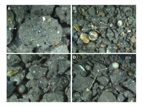
Figure 6: Parts of collected ejecta produced at four impact experiments. In each case we found multimineralic large fragments ( $\alpha$ ), monomineralic fragments ( $\beta$ ) and individual inclusions that were attached to a small amount of CM matrix.
