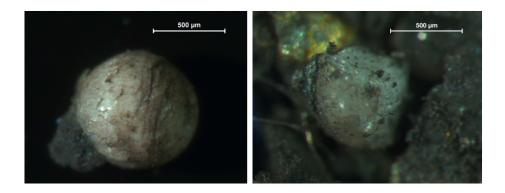
Figure 7: Examples of a shocked, shuttered and broken spheres that were used as inclusions in the CM matrix.
