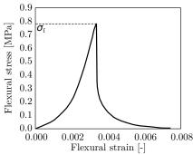
Figure 2: Typical stress-strain curves with indication of compression strength  $\sigma_c$  and elastic modulus  $E_c$  (left) and the flexural strength  $\sigma_f$  (right).
