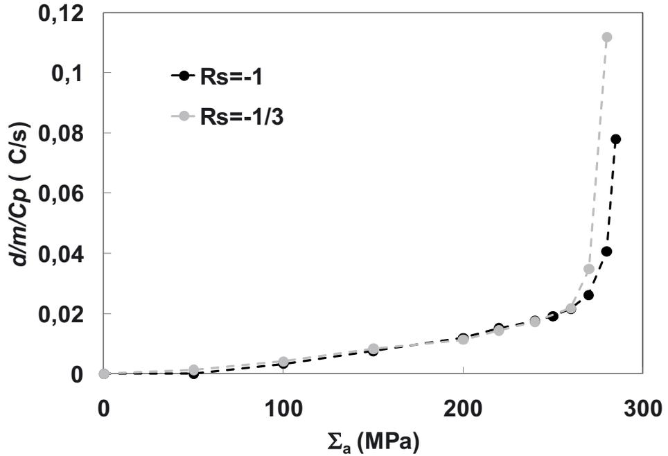
Fig. 1. Experimental heating curves obtained for a ferritic steel having precipitates (HSLA) for two loading ratio  $R_s$ .
