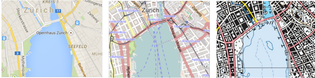
Figure 4: Three multi-scale maps at the same zoom level (respectively GoogleMaps, OSM, Swisstopo), on the same region: there is no consensus on the content (theme, abstraction, granularity) of a topographic map.
