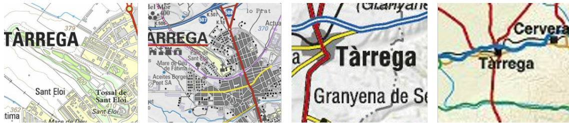
Figure 15: The proposed four abstraction levels of buildings in multi-scale maps: individual building, block, built-up area, and point.
