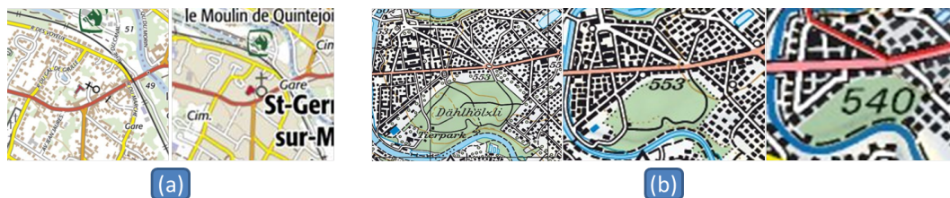
Figure 22: (a) The red center building is preserved as landmark at the urban area LoA (source: IGN Scan Express). (b) the typification of buildings makes building generalization progressive (source: SwissTopo).
