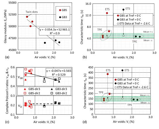
Fig. 11. Complex Young's modulus and complex Poisson's ratios constants of tested samples as a function of air-void content: (a) glassy Young's modulus ( $E_0$ ); (b) Young's modulus characteristic time at  $T_{\rm ref}$  ( $\tau_{0E}$ ); (c) glassy Poisson's ratios  $\nu_0$  and  $\nu_{00}$  in Directions 2 and 3, respectively; and (d) Poisson's ratios characteristic time at  $T_{\rm ref}$  ( $\tau_{0\nu}$ ).
