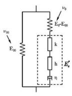
Fig. 1. Analogical representation of 2S2P1D model.
