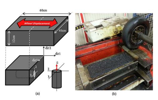
Fig. 2. Diagram of tested specimen production: (a) bituminous mixture specimen obtained from slab; and (b) French LPC compactor used to make bituminous mixture slabs.
