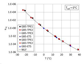
**Fig. 8.** Shift factors  $(a_{TE})$  for all tested samples of GB3 and GB5 mixtures. The line represents the WLF fitting curve [Eq. (10)].
