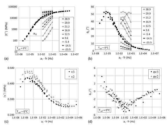
Fig. 6. Experimental results for sample GB3-TPE1: (a)  $|E^*|$  isotherms and master curves; (b)  $\phi_E$  isotherms and master curves; (c) master curves of  $|\nu^*|$ ; and (d) master curves of  $\phi_{\nu i}$ .
