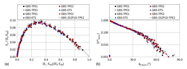
**Fig. 10.** Normalized complex Young's modulus data of GB3 and GB5 mixtures: (a) Cole-Cole plane; and (b) Black diagram. The line represents the 2S2P1D simulation [Eqs. (7) and (11)].
