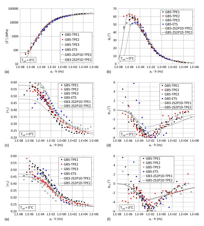
**Fig. 9.** Master curves for GB5 tested samples (data points) and 2S2P1D simulation curves for GB5-TPE2 (solid line) and GB3-TPE1 (dashed lines): (a) norm of complex modulus; (b) phase angles of complex modulus; (c) norm of complex Poisson's ratio  $\nu_2^*$ ; (d) phase angle of complex Poisson's ratios  $\nu_3^*$ ; (e) norm of complex Poisson's ratio  $\nu_3^*$ ; and (f) phase angles of complex Poisson's ratios  $\nu_3^*$ .
