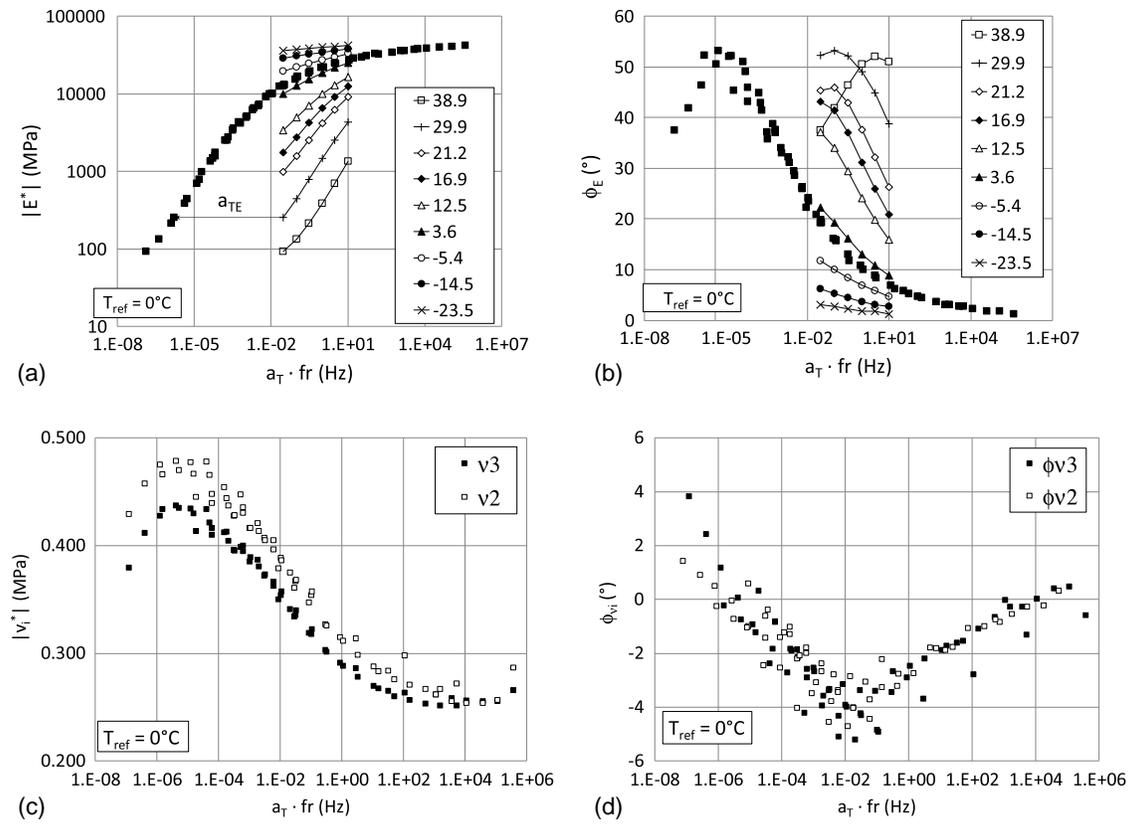
**Fig. 6.** Experimental results for sample GB3-TPE1: (a)  $|E^*|$  isotherms and master curves; (b)  $\phi_E$  isotherms and master curves; (c) master curves of  $|\nu_i^*|$ ; and (d) master curves of  $\phi_{\nu_i}$ .
