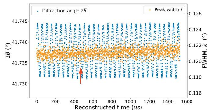
**Figure 12** Reconstructed cycles showing the effect of fatigue loading in terms of  $2\bar{\theta}$  (blue) and peak width ( $k$ , orange) versus reconstructed time for the (311) plane and a displacement amplitude of  $3.5 \mu\text{m}$ . The red arrow points out the beginning of a particular cycle ( $t = 470 \text{ s}$ ) that is used in the following images and discussion (see text for details).
