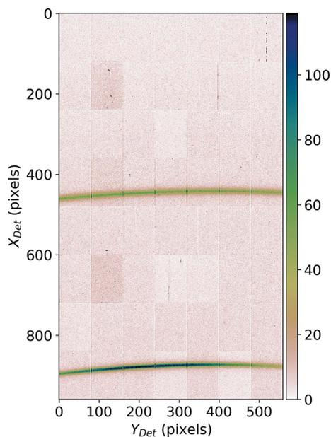
**Figure 5** The raw 2D diffraction pattern of  $960 \times 560$  pixels recorded by XPAD3.2.
