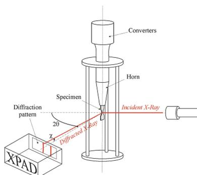
only. Ultrasonic fatigue machines typically operate at 20 kHz and allow generating so-called S/N curves (stress amplitude versus the number of cycles at failure) in the VHCF domain.
