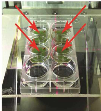
Figure 1. Dosimetry protocol takes in place on the SARRP irradiator
