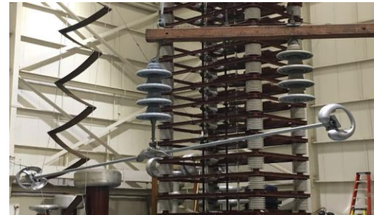
Figure 12: Up and Down Withstand Test Setup
