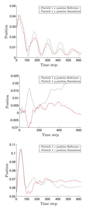
Fig. 10 Integration of the sloshing movement versus ground truth. Initial velocity 0.175 m/s. Figures represent, respectively from top to bottom, the displacement of particle number 1 along *x*, *y* and *z* coordinates
