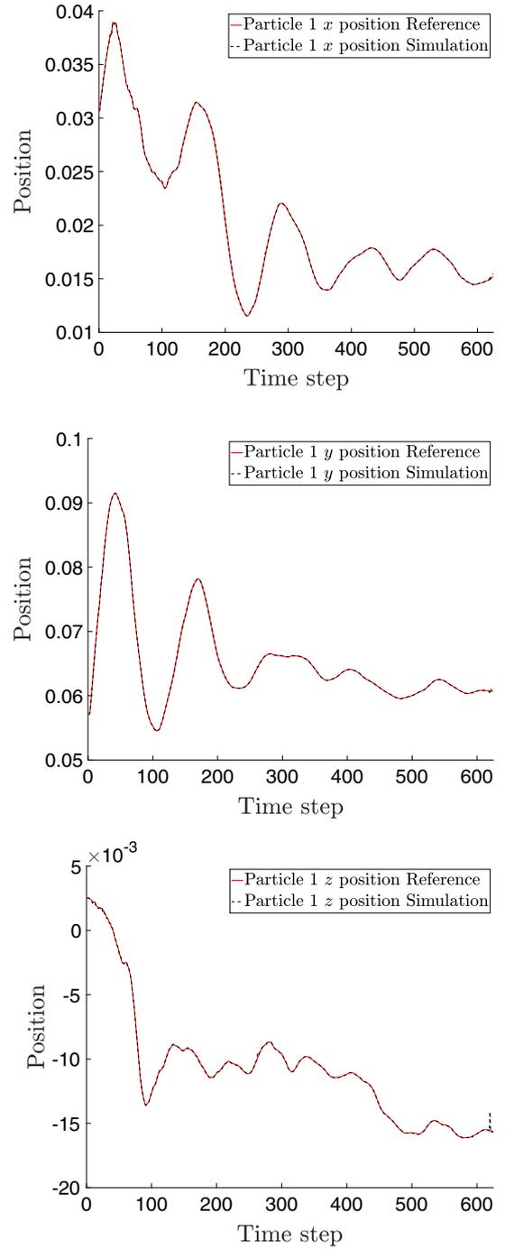
**Fig. 7** LLE-based reconstruction of the trajectory of one particular particle (evolution of coordinates  $x$ ,  $y$  and  $z$  along time) versus pseudo-experimental results. Initial velocity 0.15 m/s
