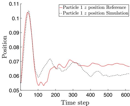
**Fig. 10** Integration of the sloshing movement versus ground truth. Initial velocity 0.175 m/s. Figures represent, respectively from top to bottom, the displacement of particle number 1 along  $x$ ,  $y$  and  $z$  coordinates
